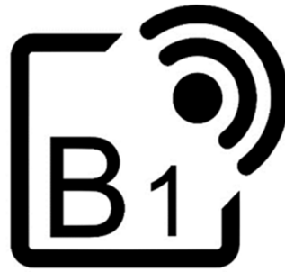
Figure 22: RFID emblem for RTIs according to ISO/IEC 17364
