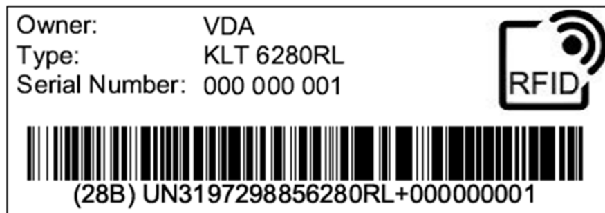
Figure 23: Example label with 1D barcode symbol and HRI.
